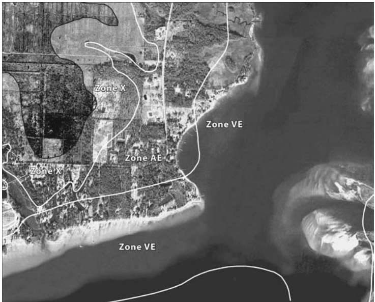
Figure 1.4. Observed surge high-water line (solid gray) versus those predicted (solid white) for Hurricane Ivan. Zone VE: Area subject to inundation by the 1%-annual-chance flood event with additional hazards due to storm-induced velocity wave action. Zone AE: Area subject to inundation by the 1%-annual-chance flood event determined by detailed methods. Zone X: Area of minimal flood hazard higher than the elevation of the 0.2%-annual-chance flood. See figure 1.2 for location. (From http://www.fema.gov/pdf/hazard/flood/recovery_data/ivan/maps/K33.pdf .)
