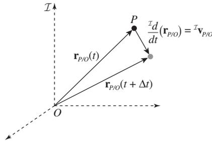
**Figure 1.4** Velocity  ${}^{\mathcal{I}}\mathbf{v}_{P/O}$  is the instantaneous rate of change of position  $\mathbf{r}_{P/O}$  with respect to frame  $\mathcal{I}$ . That is,  ${}^{\mathcal{I}}\mathbf{v}_{P/O} = (\mathbf{r}_{P/O}(t + \Delta t) - \mathbf{r}_{P/O}(t))/\Delta t$ , in the limit  $\Delta t \rightarrow 0$ .
