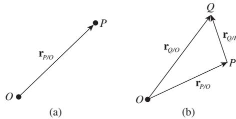
**Figure 1.1** (a) Vector  $\mathbf{r}_{P/O}$  from reference point  $O$  to point  $P$  represents the position of the point  $P$  relative to  $O$ . (b) The addition of two vectors,  $\mathbf{r}_{P/O}$  and  $\mathbf{r}_{Q/P}$ , to get the resultant vector  $\mathbf{r}_{Q/O}$ .
