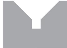
The same problem arises with the conical centre used to support the end of a long slender piece of work at the end of a lathe. It is easy enough to turn the conical centre itself, but it is extremely difficult to drill the matching hole in the workpiece. As with vee-blocks the solution is not to attempt to drill to a point, but to remove the point altogether with a special centre drill so that the cone can sit properly, without shaking.
