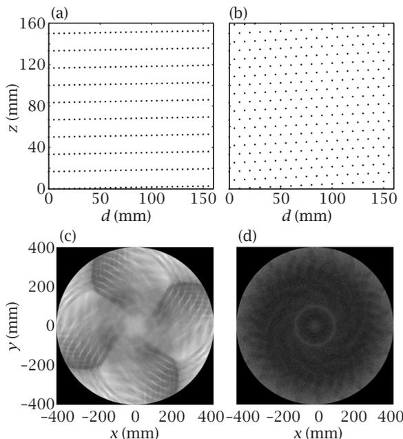
**Figure 2** (a), (b) Two multithreaded helix source firing sequences; (b) a lattice on the cylinder of source positions. (c), (d) The number of rays intersecting each voxel for the firing orders above. The second sequence (b), (d) has more uniform coverage of the cylinder and produces a more uniform distribution of rays.
