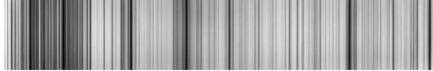
Figure 1.1: Spectroscopic image of light from the sun. The black ‘Fraunhofer lines’ correspond to various differences of eigenvalues of the Schrödinger operator for atoms such as H, Fe, Ca, Na, and Mg that are present in the solar atmosphere. Light at these frequencies resonates with frequencies of the transitions between energy states in these atoms and is absorbed. Spectroscopic measurements such as these are a crucial tool in chemical analysis, not only of astronomical bodies, and by making possible the measurement of redshifts of distant galaxies, they led to the discovery of the expanding universe. Original image courtesy of the Observatories of the Carnegie Institution of Washington.
